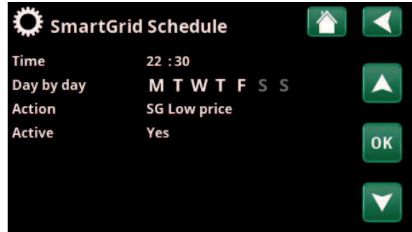
Menu: "Installer/Settings/SmartGrid schedule".
