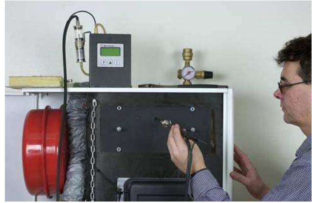
2. A space in the front part of the boiler is provided in the cleaning door to proceed to measurements.
